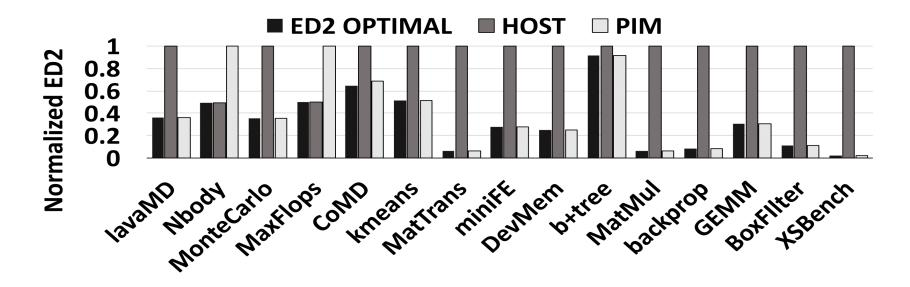
Addition of PIMs to a heterogeneous node architecture can yield high energy efficiency even compared to applications running on host running at lower DVFS states
