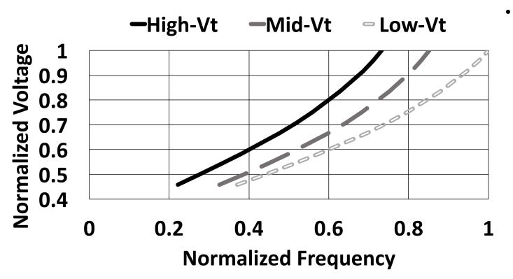
We pick a V/f curve for a 14nm chip similar to Hawaii for a specific type of transistors
