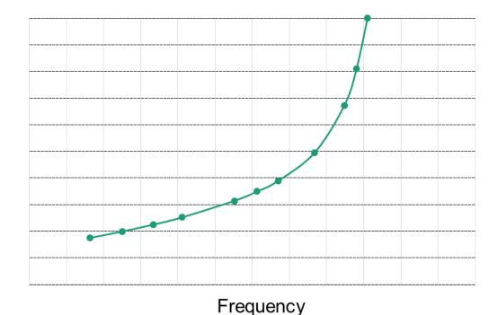
• The curve represents how static power changes with frequency for a circuit built of 50/50 HVT/MVT devices
