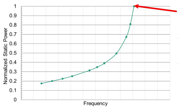
Pick a baseline point and estimate the leakage power at this particular V/f point
