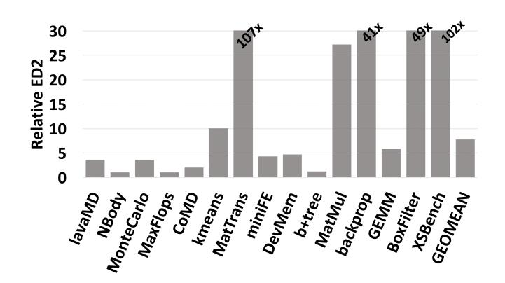
Minimum achievable ED<sup>2</sup> on a hybrid host/PIMsystem with DVFS to a host/PIM system without DVFS (running on highest DVFS state) and host/PIM co-optimization
